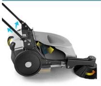
The lateral wheel of the sweeper in addition to activating the main brush, also activates a drive shaft connected to a fan. The ratio between the wheel and drive shaft creates strong suction, which picks up dust and channels it towards the filter.
