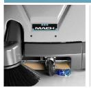
The flap fitted to the front of the machine can be lifted when collecting bulkier debris.
