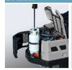
The petrol version (MACH 6 HGK LPG) can also be used with LPG gas, meaning it's possible to work in both interior and exterior environments with the same machine.
