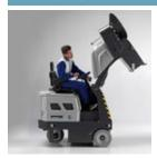
The hopper is positioned at the front of the machine and can be lifted, via a hydraulic high dump system, to a maximum height of 1.565 mm. The hopper is floating, and self regulates to facilitate the pickup of bulkier debris.
