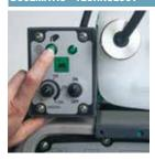
The DoseMatic® kit (optional) allows real time adjustment of the percentage of detergent being delivered to the floor, for optimum results, without waste.
