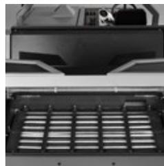
Antistatic filter, washable, with an automatic shaking system. Delivers high performance filtering that is maintained over time.
