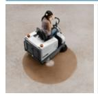
The compact MACH 2 sweeper has a reduced turning radius (950 mm), which enables cleaning in tight spaces which are difficult to access.
