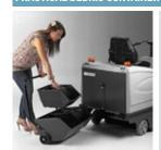
Positioned at the rear of the machine the debris container has a loading capacity of 63 liters [83 Kg]. Made of steel, mounted on wheels, and fitted with a comfortable handle for easy transport and emptying. The optional lift out baskets make emptying even simpler.
