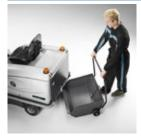
85 liters of hopper capacity is one of the key strengths of the MACH 3 PRO, allowing the sweeper to work longer before having to stop and empty. The optional lift-out baskets facilitate easy emptying.
