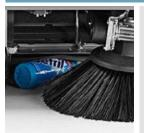
The flap fitted to the front on the machine is activated from the driver's position and allows the main brush to pick up bulkier debris
