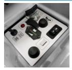
All the machines functions including the traction and control of the brushes and suction, are managed via simple and intuitive controls which are easy to access.
