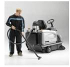
The MACH 3 PRO sweeper (EB version only) is also available with a vacuum cleaner kit. Designed for cleaning under tables, chairs, and other recesses or to reach shelving and raised surfaces.
