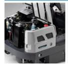
All the internal mechanical parts of the sweeper are easy access for simple maintenance operations, all the rear, side, and upper panels completely open. The batteries (EB EVOLUTION version) can be changed quickly and simply.
