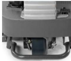
The traction motor is sealed and protected by a robust steel bumper which also incorporates an anti-tilt device. The tyre of the drive wheel is made of non-marking and anti-skid polyurethane.
