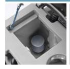
The design of the recovery tank, with a capacity of 135 L, facilitates emptying, cleaning and sanitizing operations.
