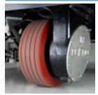
Powerful and reliable, the traction motor is vertically installed in the front part of the machine. The front wheel is driven via a gear box which is lubricated and sealed to protect it against impact, dirt, and humidity.
