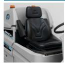
The operator's seat is equipped with weight sensors and a seat belt, it is also possible to cut off power in an emergency or during maintenance operations, guaranteeing maximum protection and safety to operators and mechanics.
